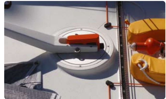
ABOVE The top of the bearing with adjustable rudder balance.
